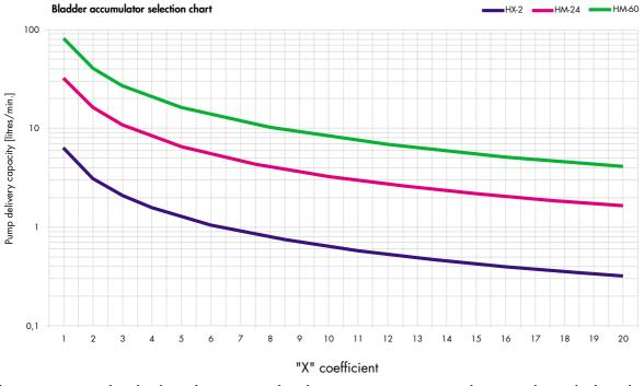
To make sizing easier, a chart has been drawn up to select the most appropriate accumulator according to both working pressure and delivery criteria. Note that the chart is based on the following hypothesis: standard precharge and 15 pump starts per hour (see p.19 to identify the "X" coefficient).
